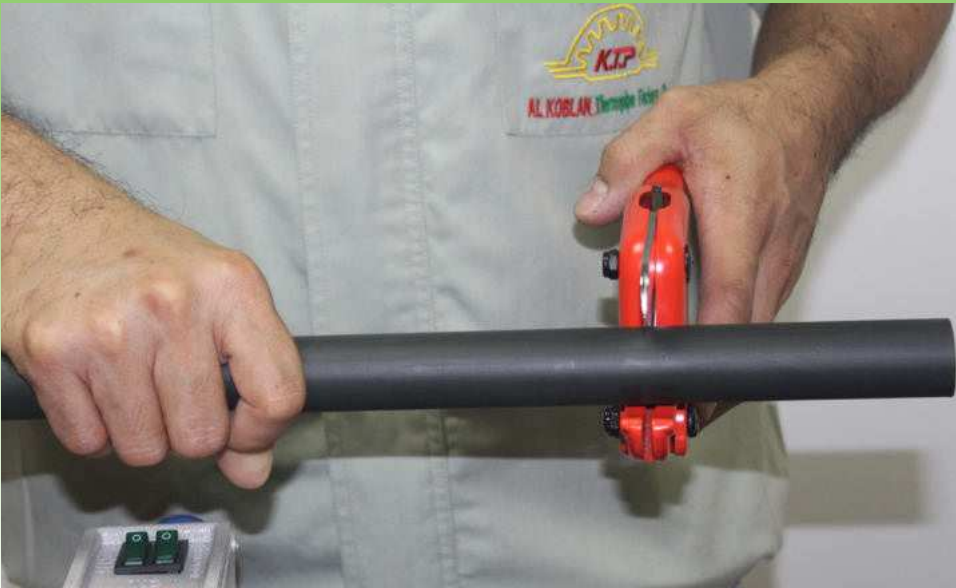
Fig. 8: PPr-PE Pipe & PPr-FG-PPr PE Pipes Cutting
