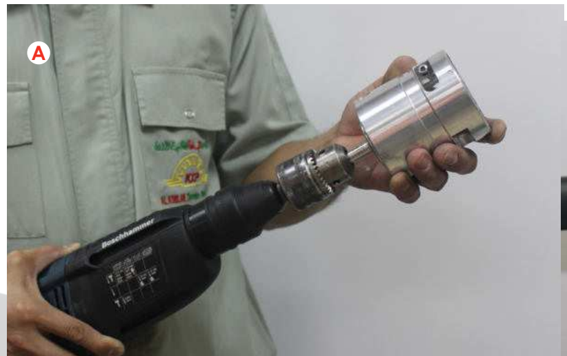
Figs. 5: Mechanical peeling process for sizes 20mm to 63mm
